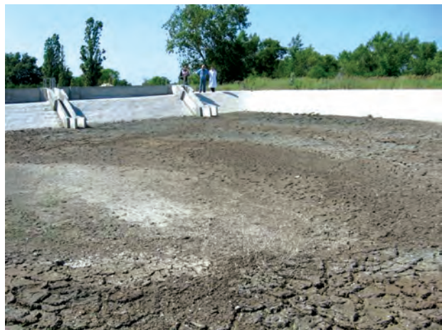
Aerobically stabilized sludge with a moisture content of 75%
