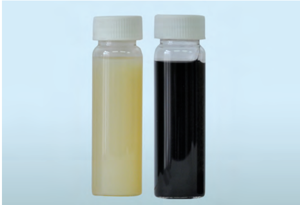
Nanofluids based on aluminum silicates (left) and carbon nanotubes (right)
