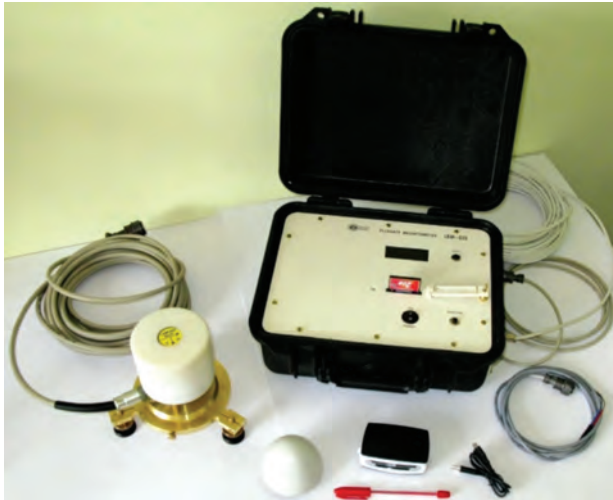
LEMI-025 reference fluxgate magnetometer with sensor, GPS antenna, and card reader
