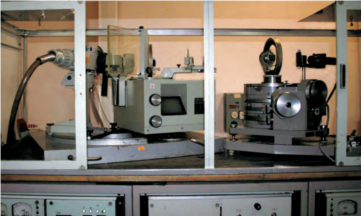
Device for nondestructive diagnosis of several types of single crystal defects
