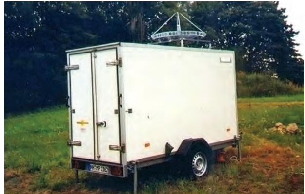
Vertically pointed meteorological radar
