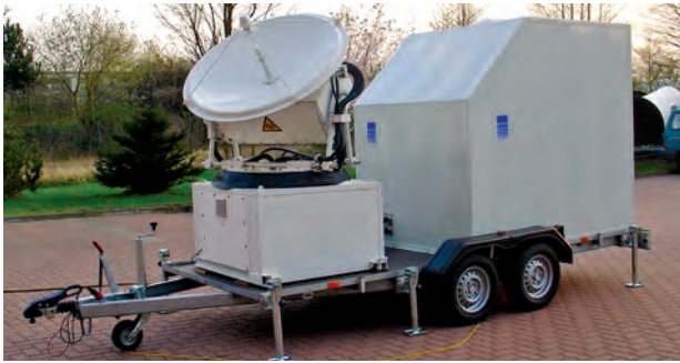
Meteorological radar with a scanning antenna
