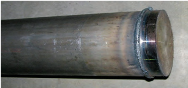
Hydraulic cylinder body, \varnothing 110 \times 7.5 mm
