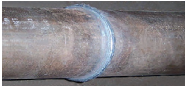
Weld joint, pipe \varnothing 120 \times 7 mm
