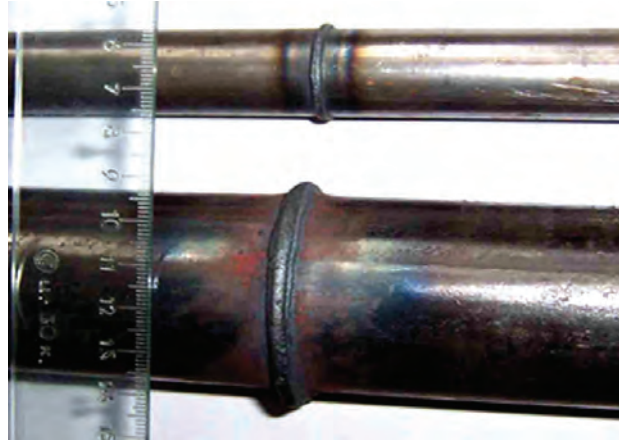
Weld joints , \varnothing 25 \times 2 mm, \varnothing 42 \times 4 mm
