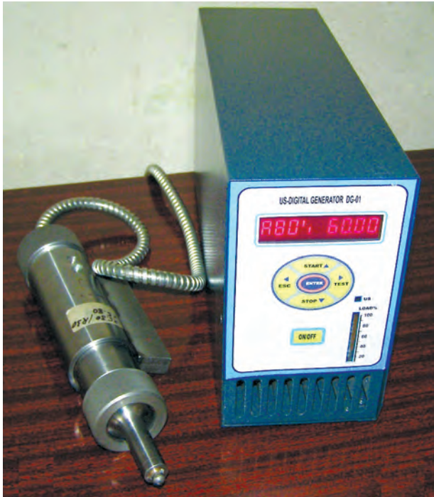
USFT equipment (an instrument with a tungsten carbide tip; US generator)
