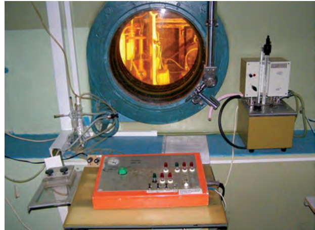
Hot cell of stationary generator for 99mTc extraction
