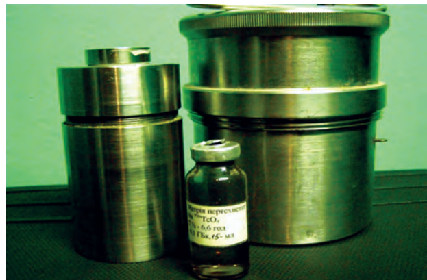
99mTc-pertechnetate and transport portable container
