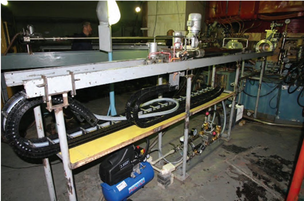
Automated installation for ^{82}\text{Sr} radionuclide production
