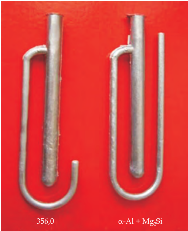
Fluidity of industrial cast 356.0 (USA) and ( \alpha -Al + Mg_2Si ) alloys
