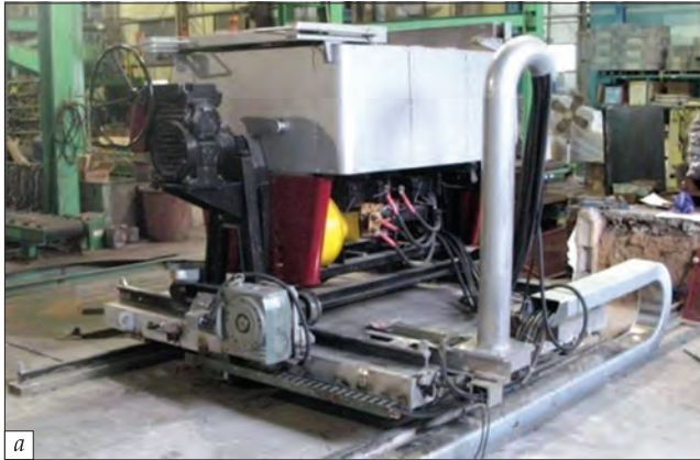
Magnetodynamic mixing-and-batching devices for aluminum alloys (a) and for cast iron and steel (b)
