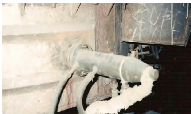
Continuous light-guide temperature control of liquid cast iron in the induction channel pouring furnace
