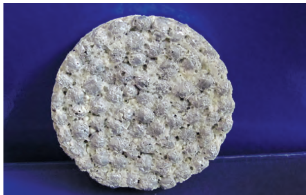
Sound absorbing panels with foamed pellets
