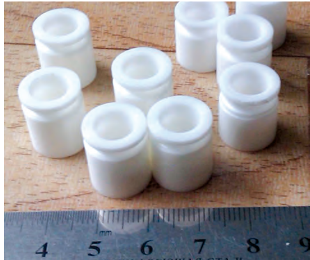
Inserts made of ZrO_2 - Al_2O_3 composite
