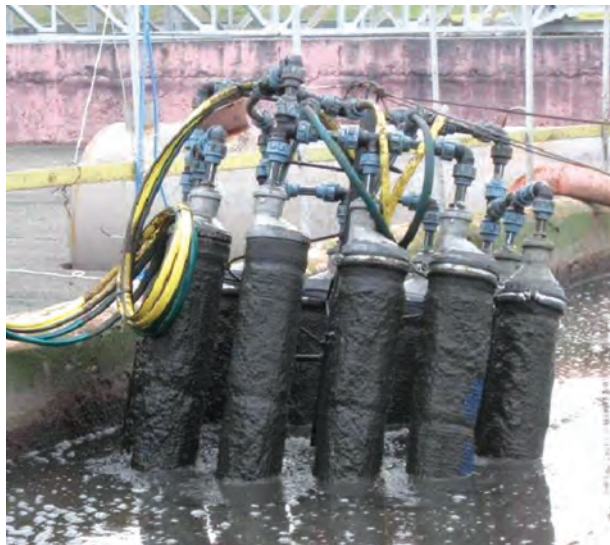
Filtering module in BSA aerobic stabilizer
