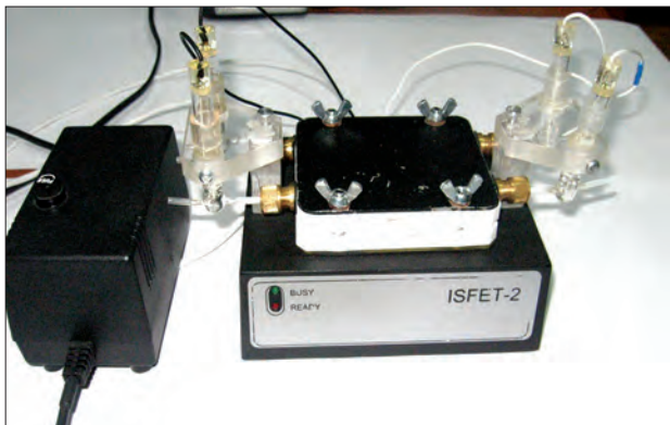
Measuring device with multibiosensor and flow-through system
