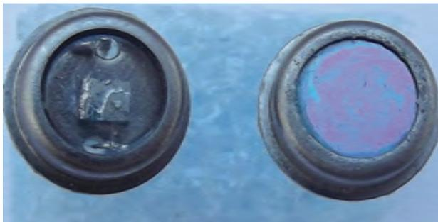
Uncooled InAs photodiode prototypes
