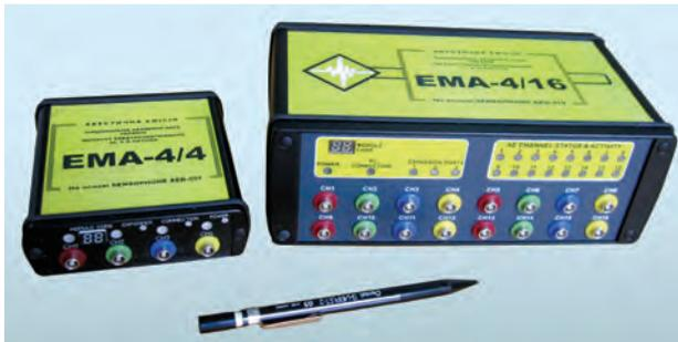
EMA-4 devices based on 4-channel and 16-channel modules
