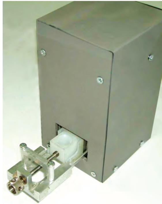
KD-3 optoelectronic colorimetric gas leak detector with a portable sensor unit
