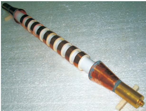
Diffraction omni-antenna for mobile communication systems
