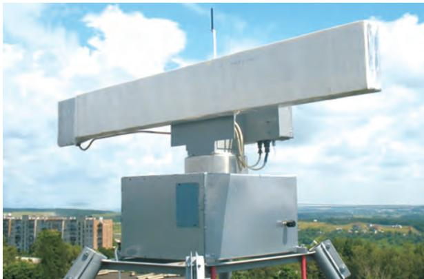
Diffraction antenna for radar systems
