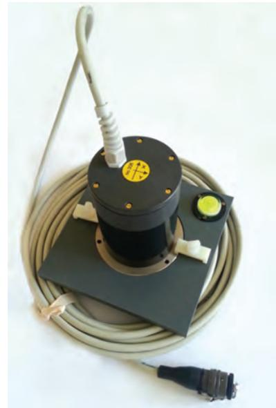
3-component fluxgate magnetometer of LEMI-424 MT station
