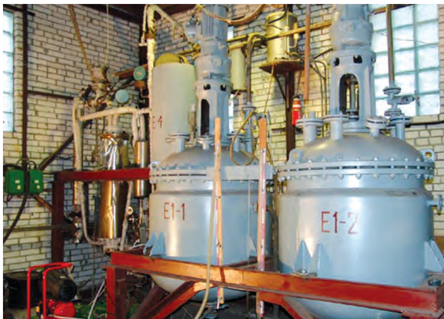
A pilot plant for producing biodiesel fuel from bio-renewable raw materials
