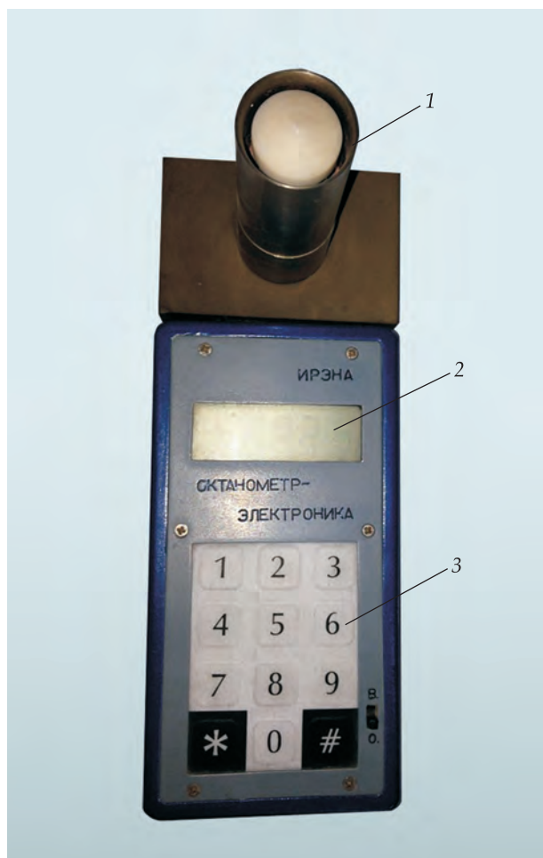
Irena portable analyzer: 1 – measuring sensor; 2 – indicator; 3 – control panel
