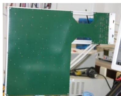
Figure 2: Example of microphone array containing 64 sensors.
