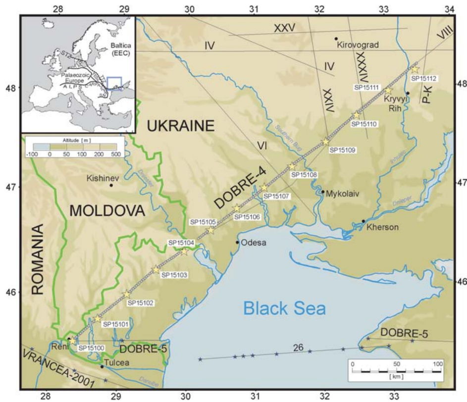
Figure 1. Location of the DOBRE-4 profile and most important previous seismic experiments in the study area. Yellow stars represent shot points; grey dots show recording stations of DSS experiment; blue stars are shot points of experiments VRANCEA-2001, DOBRE-5 and registration instruments along the profile 26 (sea part of DOBRE-5); black lines with Roman numerals are old DSS Geotraverses; green lines are state boundaries. Inset map shows the location of study area in Europe. P-K, Putivl-Kryvyi Rih profile.
