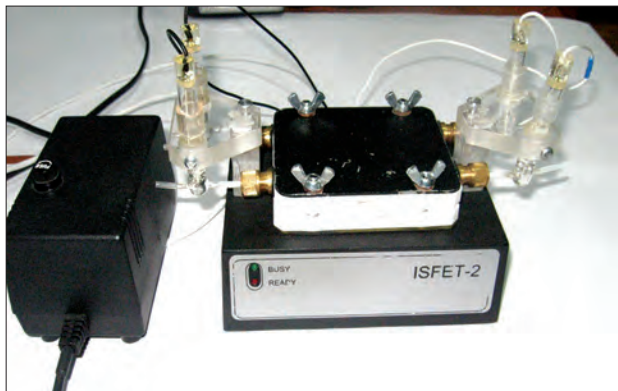
Measuring device with multibiosensor and flow-through system
