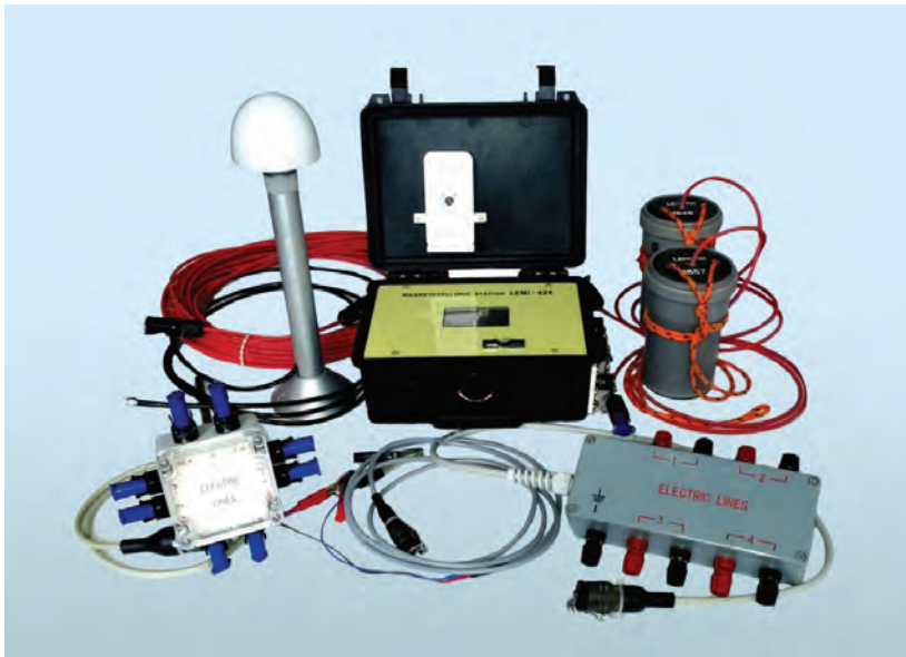
LEMI-424 MT station data logger with electrodes and complete set of field equipment
