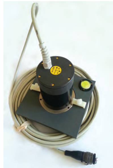
3-component fluxgate magnetometer of LEMI-424 MT station
