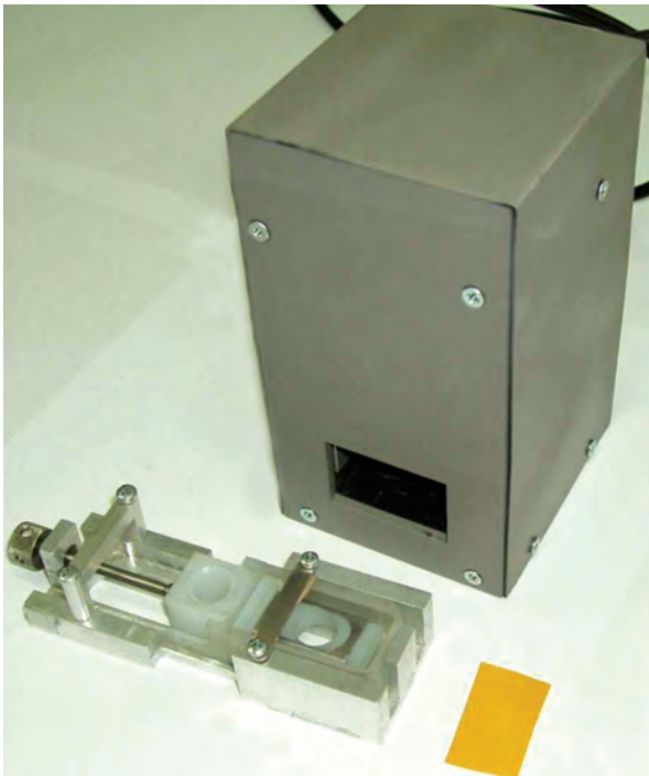
KD-3 optoelectronic colorimetric gas leak detector with a portable sensor unit
