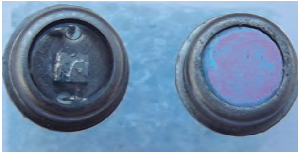
Uncooled InAs photodiode prototypes
