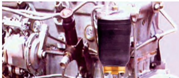
Heated fuel filter
