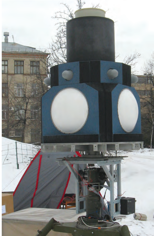
Omnidirectional coverage broadband antenna system (0.4–18 GHz)
