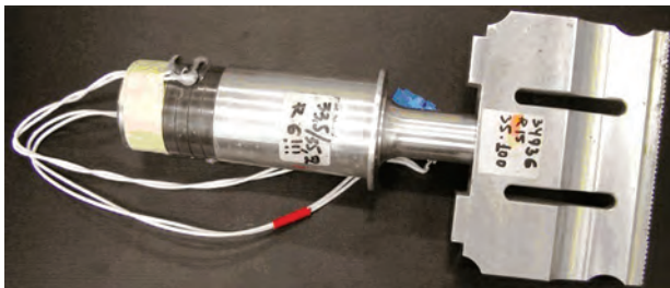
USG with a flat concentrator for welding longitudinal joints
