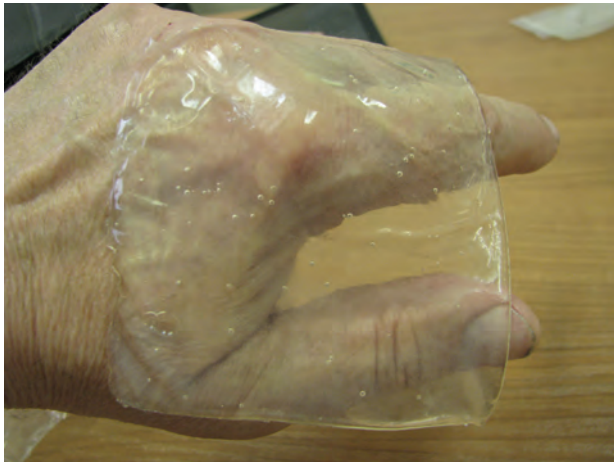
Elastic deformation of medical bandage before rupture reaches 50–100%
