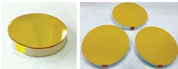
Alpha and alpha-beta detectors operating as counters (left), Alpha-beta detector operating as spectrometer (right)
