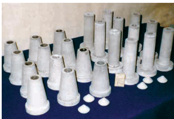
Cast stone ware that are stable in melts of salts with chlorine content
