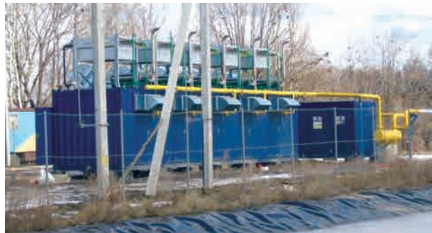
Landfill gas processing complex with a capacity of 1 MW
