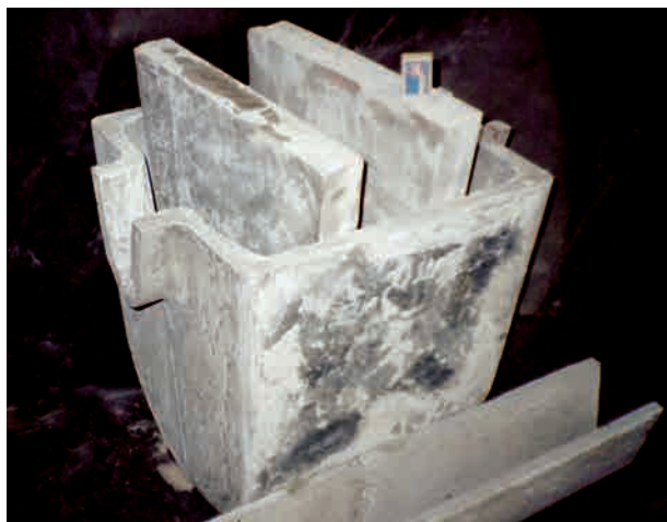
Intermediate ladle for melting high-purity aluminum, made with the use of the developed technology
