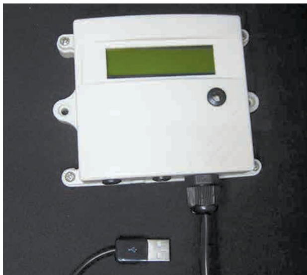
Measuring module of the air pollution monitoring system
