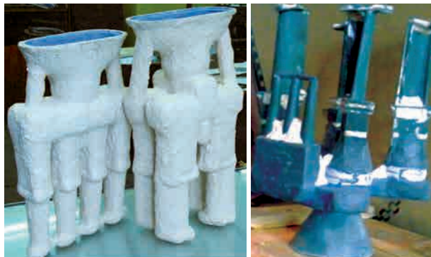
Ceramic mold obtained from a corundum-based mix modified with aluminum powder (left), and blade blocks manufactured at Zoria – Mashproekt gas turbine plant
