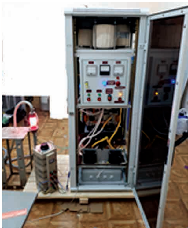
Plasma chemical plant for deep utilization of liquid radioactive waste
