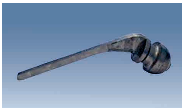
Ti and Zr castings produced by the electron-beam technology
