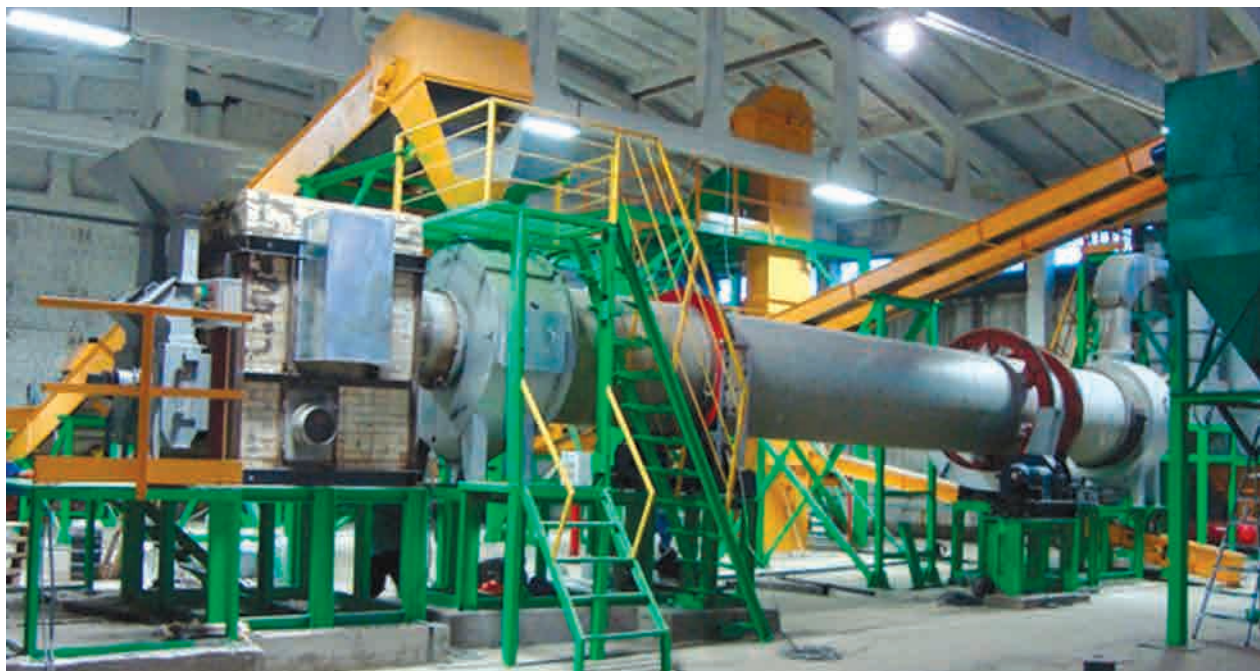
Heat generator on a drum dryer of mineral fertilizers (Berezan)
