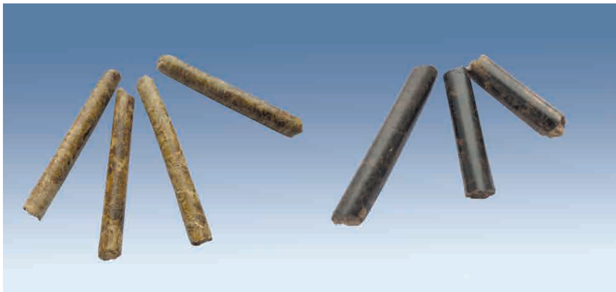
Fuel pellets (pine wood) with surface (left) and bulk (right) polymerization of biomass
