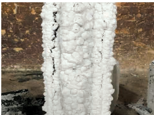
Steel pillar protected by the fire-retardant coating: before and after the fire tests
