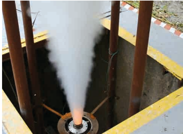
Bench for studying monofuel detonation devices and for conducting fire tests of solid propellant rocket engines
