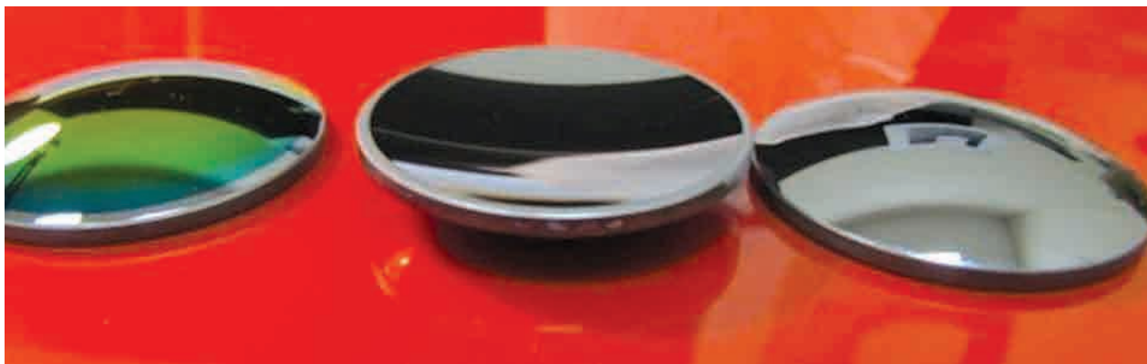
Germanium plates (a wedge and lenses) coated with \text{Ge}-\text{ZnS}-\text{B}_2\text{O}_3 material
