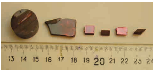
\text{TlGaSe}_2 single crystals and prepared oriented samples with faces perpendicular to various crystallographic directions
