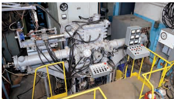
Plasma induction plant for growing single crystals of refractory metals
