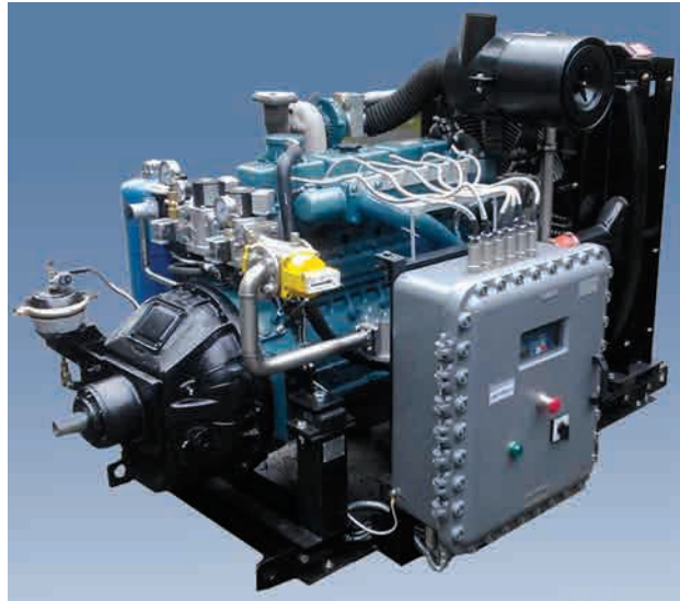
Drive motor of the compressor unit operating on natural gas (power 120 kW)
