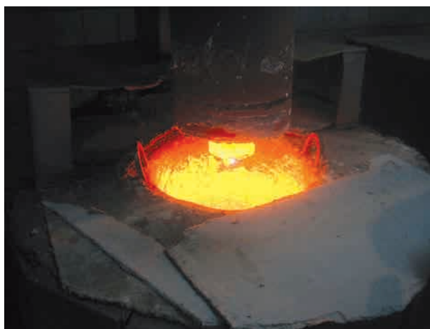
Immersing a plasma jet into the melt for refining
