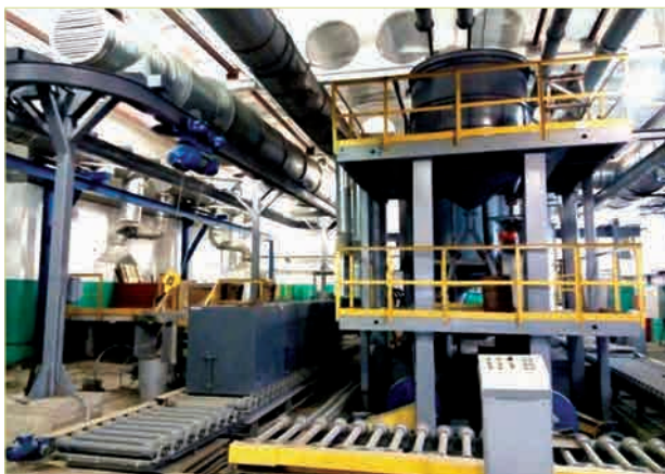
Automated casting complex for the lost foam technology implementation with 3000 ton/year capacity
