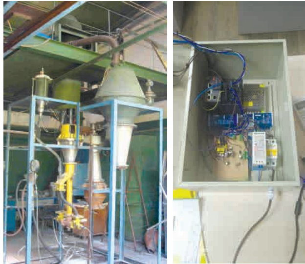
Jet mill with control system (left) Mill load control unit (right)
