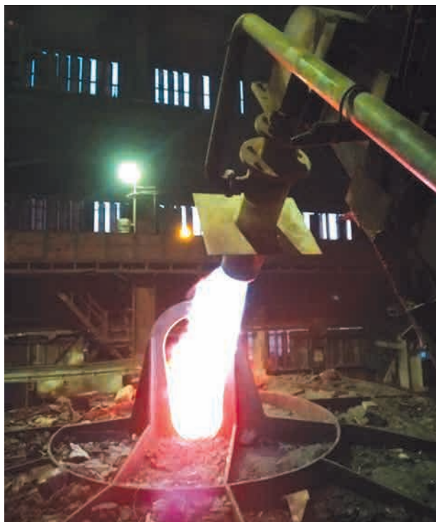
High-speed gas burner GNB-1500 before immersion into a 250-ton bucket
