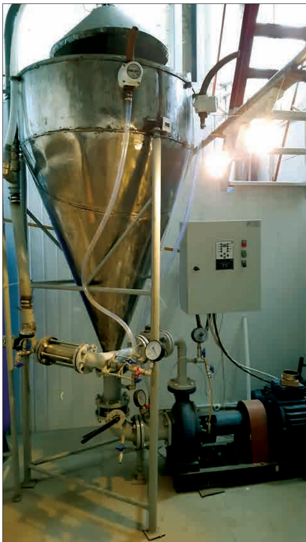
Industrial rotor-type aeration-and-oxidation plant
