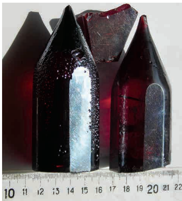
Proustite ( \text{Ag}_3\text{AsS}_3 ) single crystals
