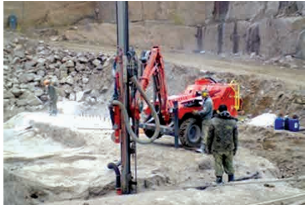
Technology for block separation from the rock mass: drilling of holes in the block
