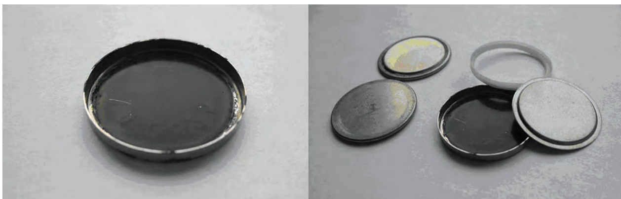
Film of nanostructured composite material (left) electrodeposited on the inner surface of lithium-ion battery body and battery components (right)
