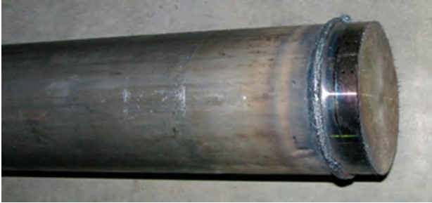
Hydraulic cylinder body, \varnothing 110 \times 7.5 mm
