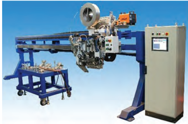
Narrow-gap argon titan welding equipment with magnetocontrollable arc
