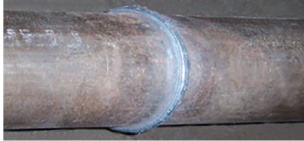
Weld joint, pipe \varnothing 120 \times 7 mm
