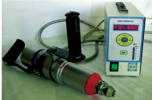
Equipment for UIT of metallic products (an impact instrument and USG)
