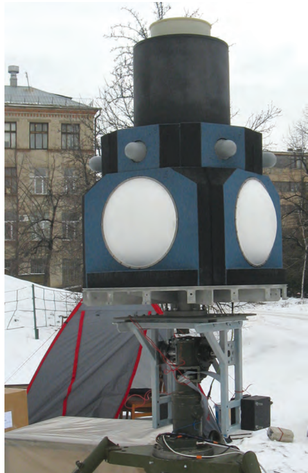
Omnidirectional coverage broadband antenna system (0.4–18 GHz)
