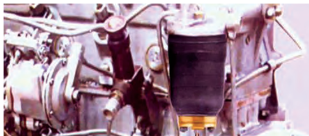
Heated fuel filter
