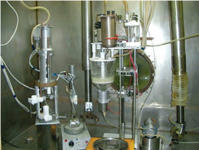
Plant for Mo-Zr gel synthesis
