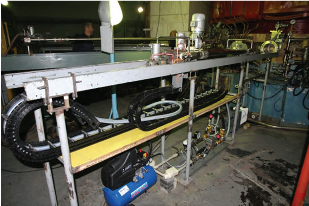
Automated installation for ^{82}\text{Sr} radionuclide production
