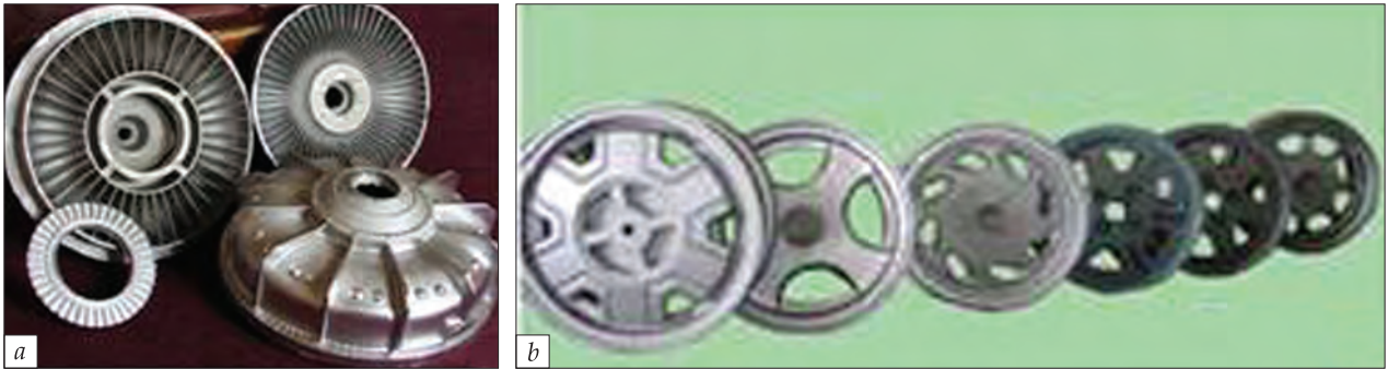
Set of hydraulic clutch components (a) and car wheels (b) obtained by the low-pressure casting method using ALUT-3 machine
