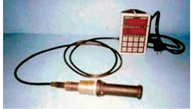
STGEACI device for rapid thermographic analysis of cast iron
