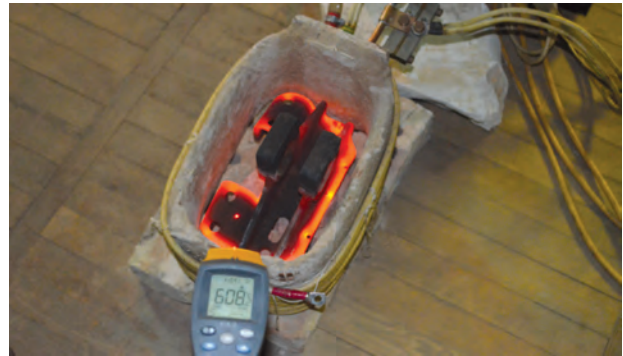
Heating of a cast-iron stop shoe of subway car reduction gear
