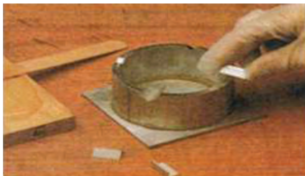
Steel to steel adhesive bonding
