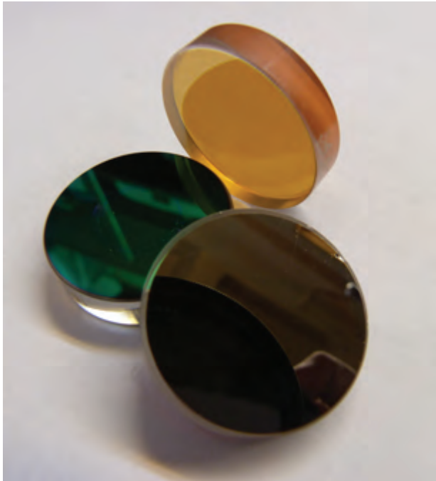
Specimens of coatings obtained from Ge - ZnS (brown color); Ge - ZnO (orange color); refined ZnS/Cr (green-blue color) on quartz substrates
