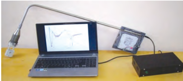
STECS-CI device for rapid thermodynamic control of graphite form in cast iron
