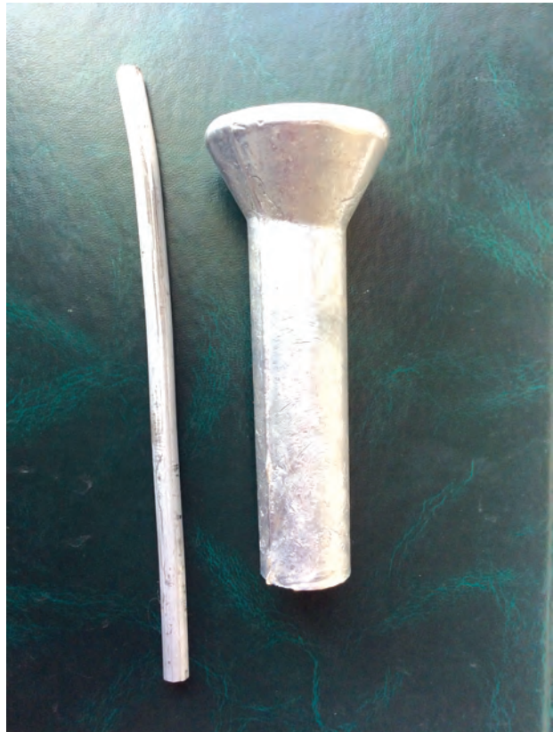
Ingot and rod obtained by the extrusion method
