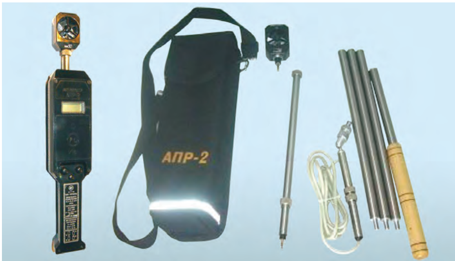
Complete set of APR-2 anemometer (left), measurements at a height of up to 5 meters (on right)
