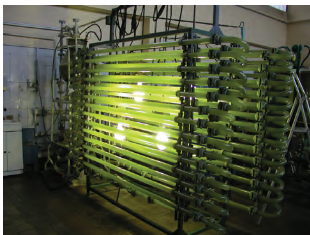
Closed-type photobioreactor for microalgae cultivation
