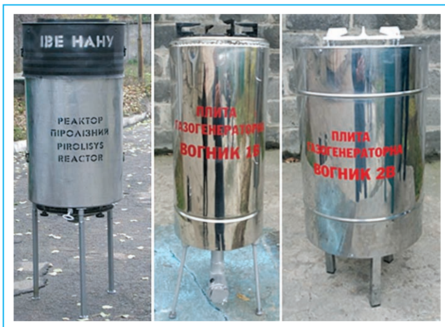
Farmer's batch-operation facility for producing bio carbon, and Vohnyk 1B and Vohnyk 2B gas-generator cooking stoves
